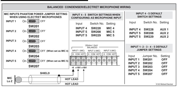
Fig. 12 - Balanced Condenser/Electret Microphone Wiring - Configuration Tables
